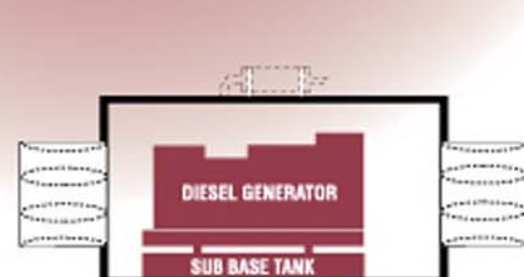
DIESEL GENERATOR ENCLOSURE WITH HORIZONTAL AIR FLOW.
